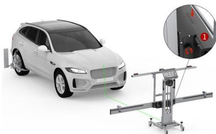
1. Adjust the left and right fine-tuning knob ① to make the laser beam of **Center laser LAC09-02** irradiates on the center of vehicle.
