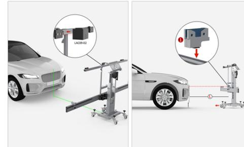
1. Install **Center laser LAC09-02** on **Mounting plate LAC09-03** and turn on the laser, place the device in front of the vehicle so that the laser beam irradiates on the center of vehicle.
